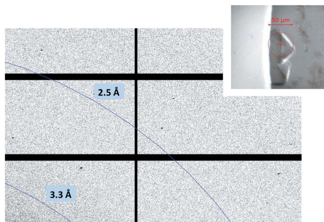
Figure 1 Example section of a diffraction image with spots extending to 2.1 Å resolution into the corners of the detector. The inset at the top right is an on-beam-axis view of two example crystals located at the edge of a crystallization drop captured during data collection. The red circle represents the full-width half-maximum of the beam profile and has been matched to the crystal size. The matching of the beam size to that of the crystal optimized the signal-to-noise ratio of the data.
